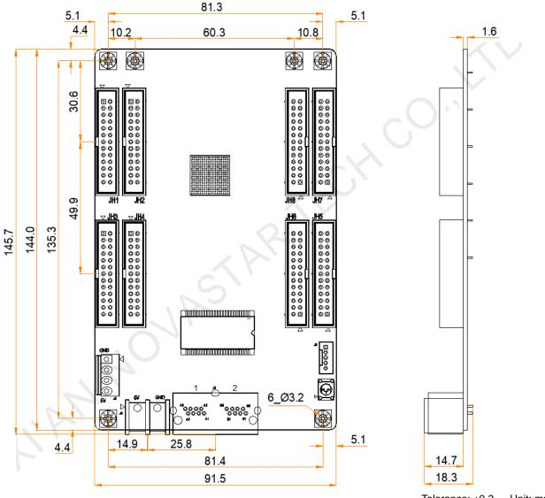
Tolerance: ±0.3 Unit: mm
