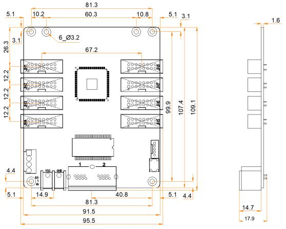
Tolerance: ±0.3 Unit: mm To make molds or trepan mounting holes, please contact NovaStar for a higher-precision structural drawing.
