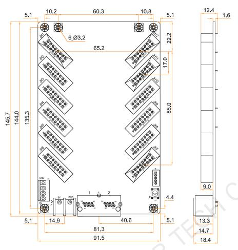
Tolerance: ±0.3 Unit: mm
