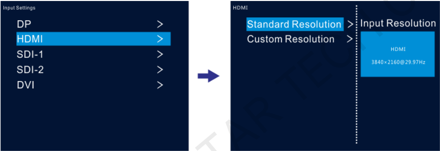
Figure 5-13 Setting input source resolution
