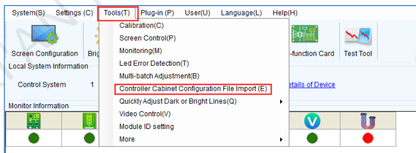
Figure 5-6 Importing controller cabinet configuration file
