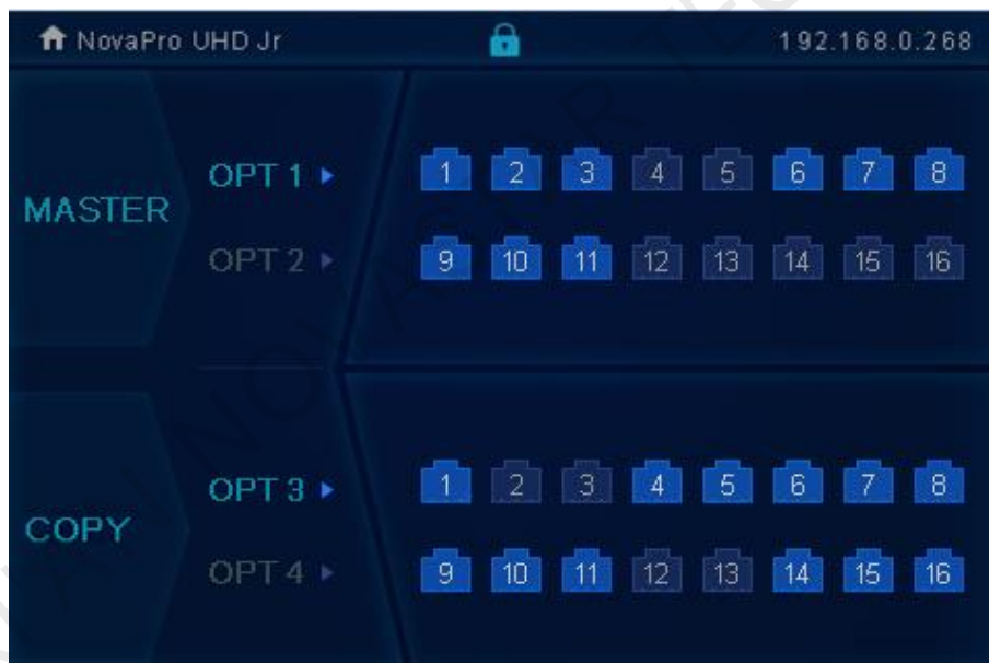
Figure 4-2 Optical fiber port statuses – Copy
