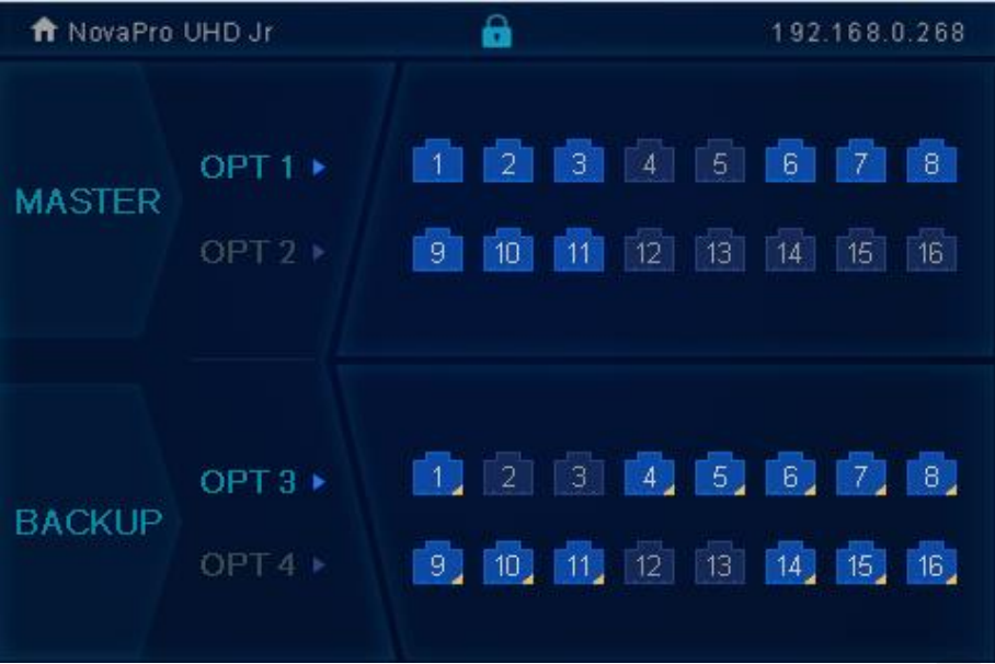
Figure 4-3 Optical fiber port statuses – Hot backup
